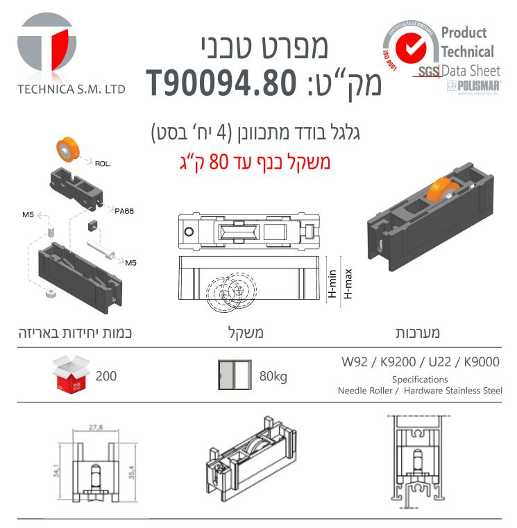
Note: In order to function properly under more extreme conditions, like salinity or high levels of humidity, the roller must be very well lubricated with extra mounting grease because the standart lubrification is for regular use. The performance of the product is assured when maintaining the conditions described in the certified laboratory test report
